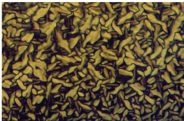
Figure 13. Optical texture of the smectic phase of L VI ·2H 2 O at 160 °C (500× magnification).
